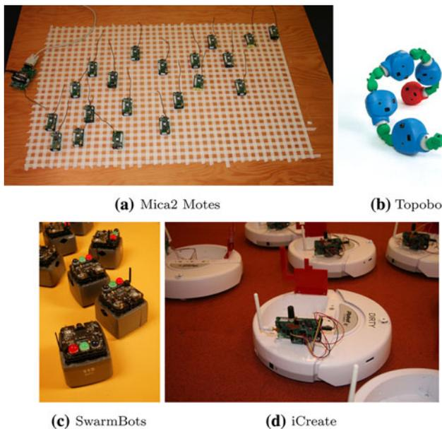
**Fig. 9** Proto's discrete kernel has been implemented on hardware for sensor networks (a), modular robotics (b), and swarm robotics (c) and (d). (Photo credit: b Hayes Raffle and Amanda Parkes and c James McLurkin and Swaine Photography)
