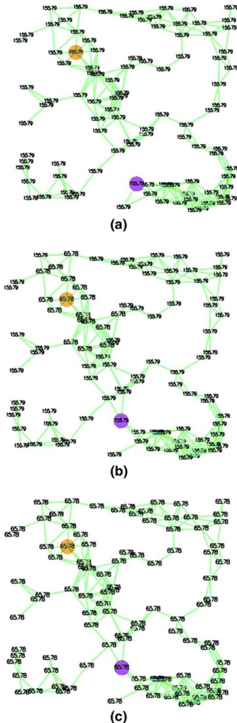
**Fig. 17** Self-healing can carry through composition: here, a program based on two instances of self-healing `distance-to` computes the distance between two regions (orange and purple) to be 156.79 m (a). When one device moves, changing the connectivity of the network and becoming much closer, the self-healing of `distance-to` quickly causes the distance estimate to adjust to the new value, 65.78 m, which begins propagating through the network (b), converging again after 24 rounds (c)
