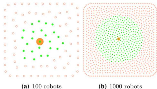
**Fig. 16** Scalability carries through composition: the `dilate` operator behaves equivalently in swarms of 100 and 1,000 robots in this example, turning on a *green light* on every robot within 0.5 m of an active light sensor (*orange disk*)
