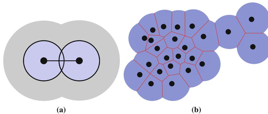
**Fig. 3** A conservative approach to determining a space that is well approximated by a discrete network (assuming unit disk communication) is to surround each device with a half-communication radius disk (**a**). The union of all such disks is a space well approximated by
