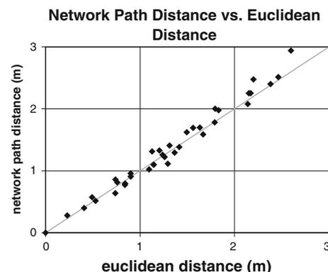
**Fig. 22** The distance estimates produced by `distance-to` executing on real robots closely approximate true distances
