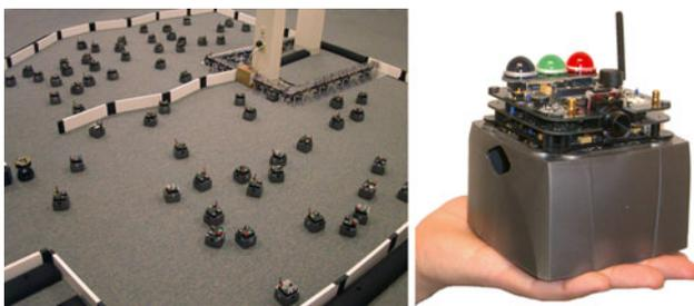
**Fig. 21** Experiments were carried out on a group of 40 iRobot SwarmBots, a platform designed for distributed algorithm development. Each SwarmBot is autonomous and is equipped with bump sensors, light sensors, and an infrared inter-robot communication and localization system
